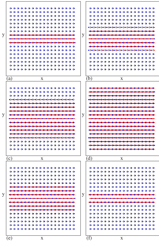
FIG. 2. (Color online) The vortex positions (dots), trajectories (lines), and pinning site locations (circles) for the system in Fig. 1(c) at F_D/F_p=0.85 during consecutive time intervals in a single large oscillation of V_x with period T . (a) At a minimum in V_x , t/T=0 , the vortices in the pin-free channel move along with vortices in one pinned row on each side of the channel. (b) At t/T=0.125 , a front of moving rows begins to propagate outwards from the pin-free channel and here three pinned rows on each side of the channel are moving. (c) Near t/T=0.25 the moving region continues to grow. (d) At t/T=0.5 the front has moved completely through the sample and all of the vortices are moving. (e) Near t/T=0.8 the moving region is contracting. (f) At t/T=1 the system returns to the minimum state of three moving rows of vortices.
